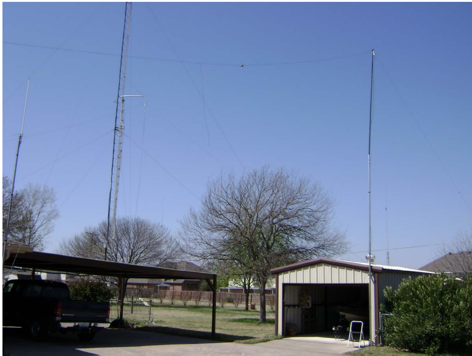
Two W8NX 80 -10 Meter Inverted Vees Spaced 32 ft and 38 ft High
