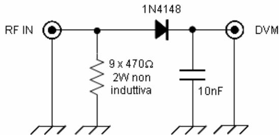
Use only non inductive resistors, do not exceed 15 W TX power with 2W resistors. A digital, high impedance DVM should be connected to the “DVM” output.
