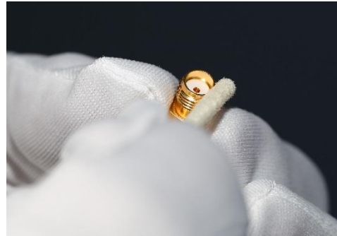
Fig. 4-3: Cleaning the thread
